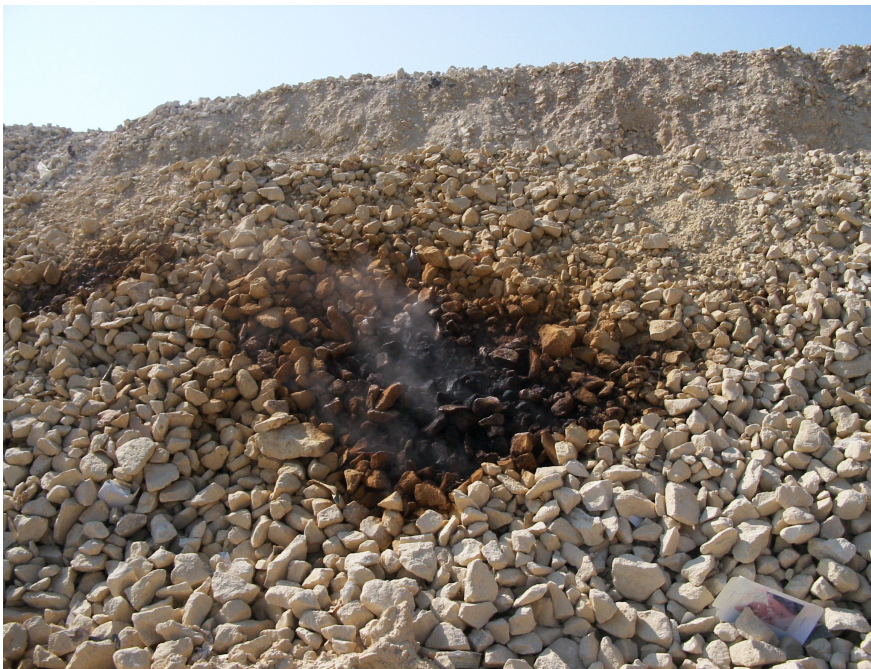
Plate 3.2: Condensate around combustion vent – Magħtab west face
